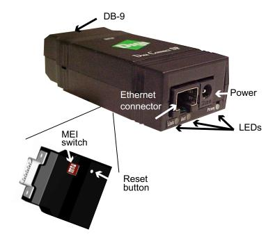
**Note** MEI switches and the Reset button are in the same location for both the Digi Connect SP and Digi Connect Wi-SP.
